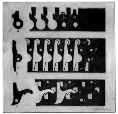
Fig. 50. Blanked Parts and Scrap, Illustrating Successive Operations
